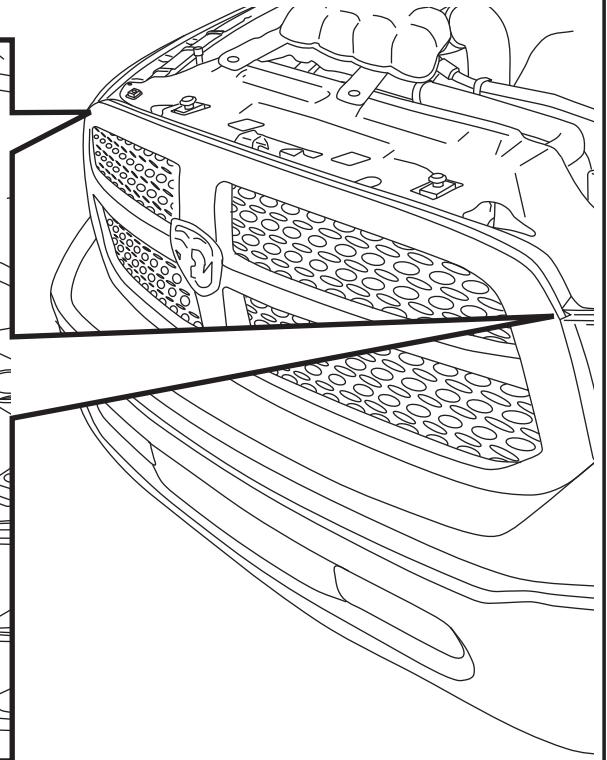
**GB** Install side pads by folding pads back behind grill and headlights, pushing pads down on each side one or two inches at a time, until they bottom out against bumper. Note: To avoid damage when removing, slide cover up from behind headlights before detaching pads.
